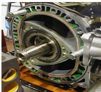
Gambar 4. Mesin Wankel Cutway.
