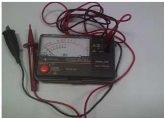
**Gambar 1. Insulation Tester**
