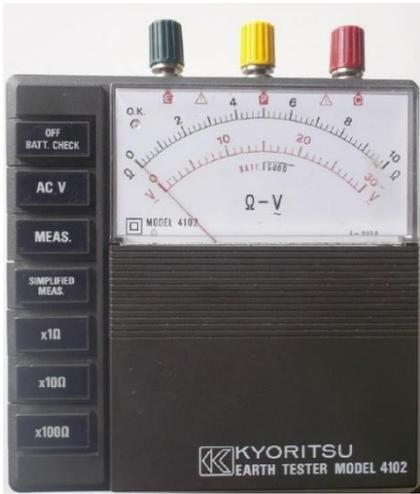
Gambar 3. Alat Ukur Earhtester Tipe 4102
