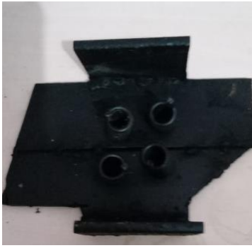
Gambar 3.2 Landasan mounting berbahan plat tebal 4 mm
