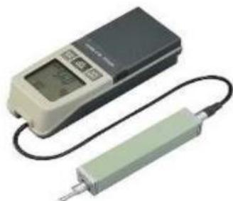
Gambar-2. Surface Test Mitutoyo
