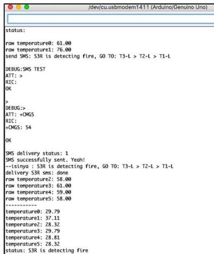
Figure 6. S3R Serial Monitor Display
