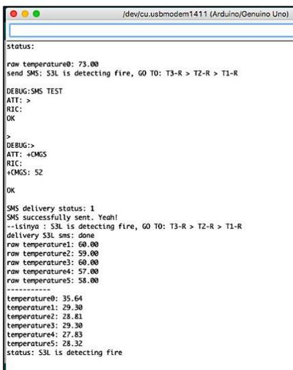
Figure 4. S3L Serial Monitor Display
