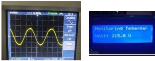
Gambar 15. Hasil output inverter+ Filter beban resistif 25 W
