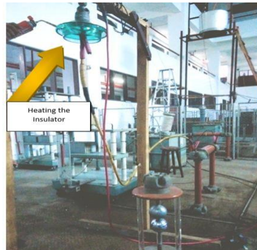
Figure 4, Heating of the Insulator
