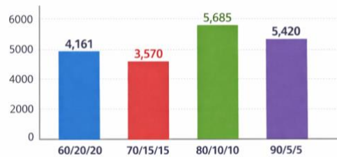
Figure 7. Average Modulus of Elasticity Graph (MPa)
