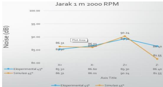
Figure 26. Graph of 2000 RPM with a distance of 1 m and an angle of 45° after using the ANC method.
