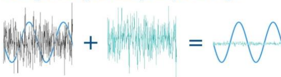
Figure 4. How Active Noise Control Works [3]
