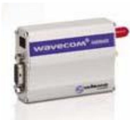
Gambar 1. Modem GSM (SR2 MOD02)
