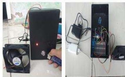
**Gambar 5. Alat sistem pendeteksi kebocoran gas LPG**
