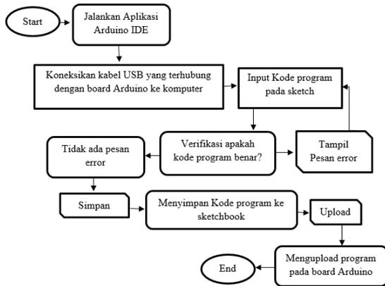
**Gambar 5. Flowchart proses upload kode program ke papan arduino**
