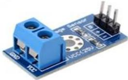
**Gambar 3. Sensor Tegangan MD0531**
