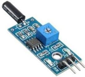
Gambar 4. Sensor getra (vibration)
