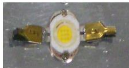
Gambar 7. Lampu LED 10 Watt
