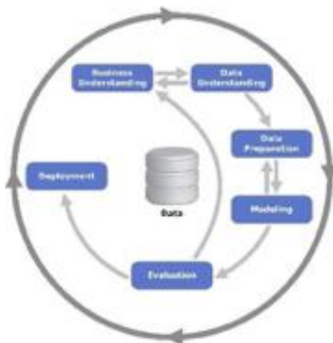
Figure 1. Research Methodology Flow Based on the CRISP-DM Approach
