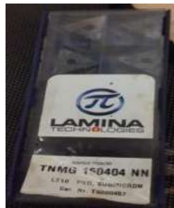
Gambar5. Pahat Insert LAMINA TNMG160404NN
