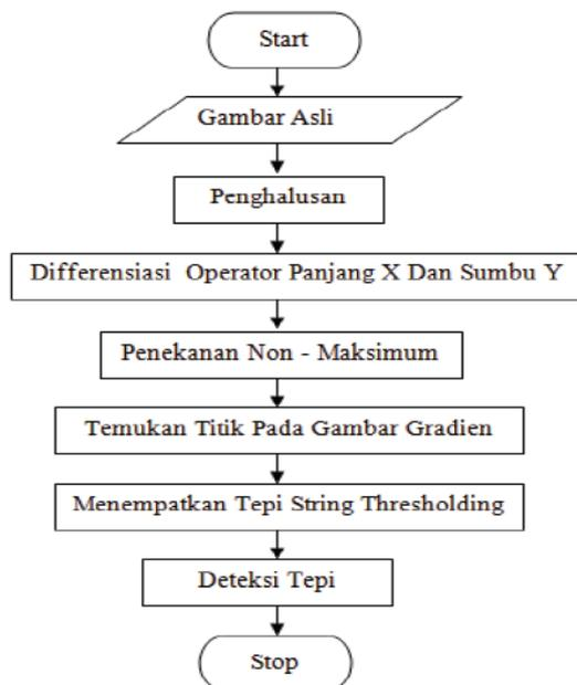
Gambar 2..Flowchart Metode Canny
